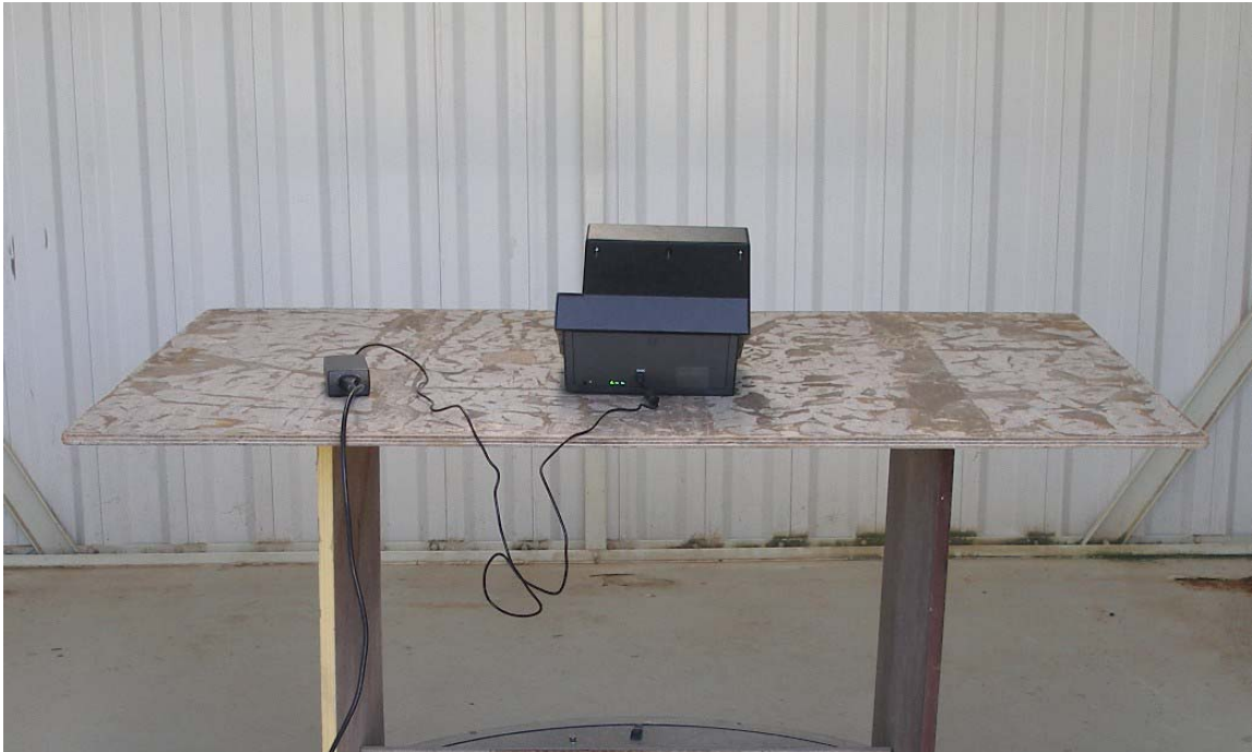
Photo # 2. Radiated emission test setup Rear view
