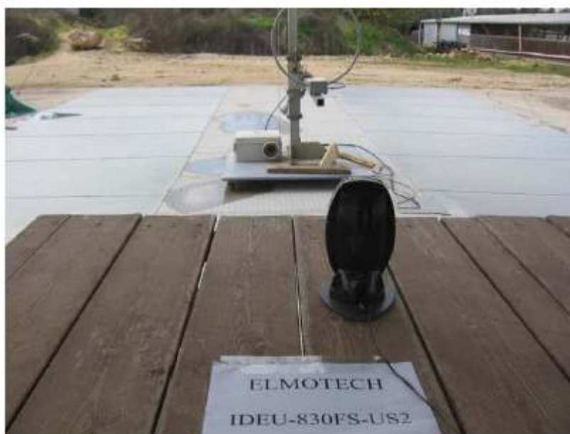
Figure 3. Radiated Emission Test 9 kHz -30 MHz
