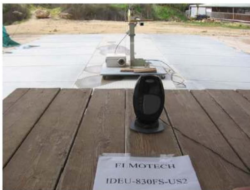
Figure 4. Radiated Emission Test 30 – 1000 MHz
