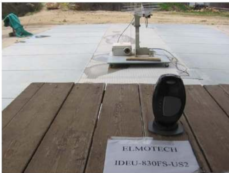
Figure 4. Radiated Emission Test 30 – 1000 MHz
