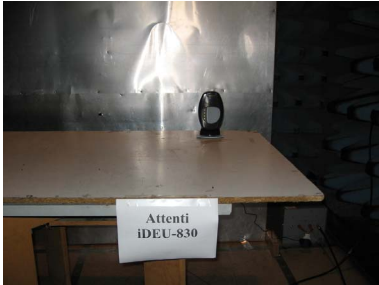
Figure 2. Conducted Emission Test
