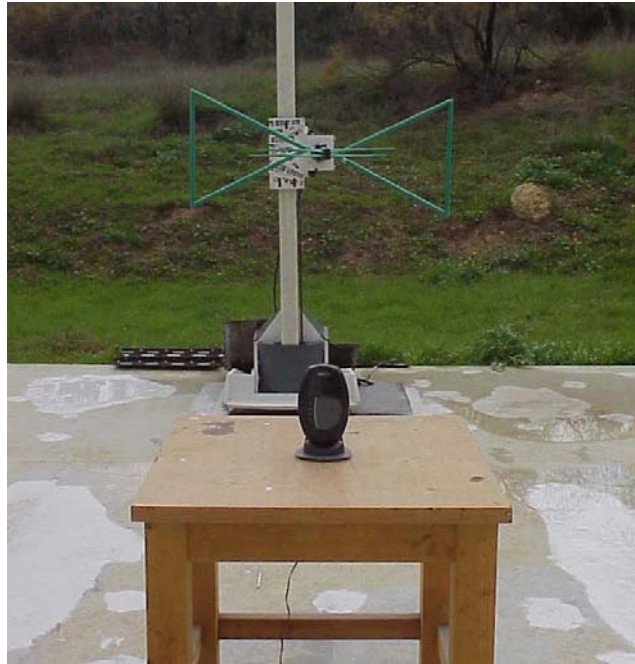
Photo 2. Spurious emissions test setup.
