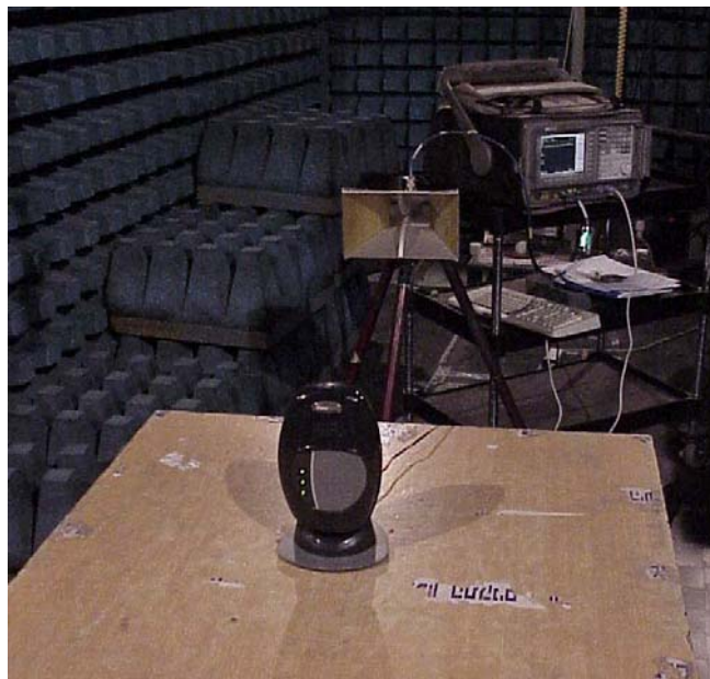
Photo 3. Spurious emissions investigation test setup.
