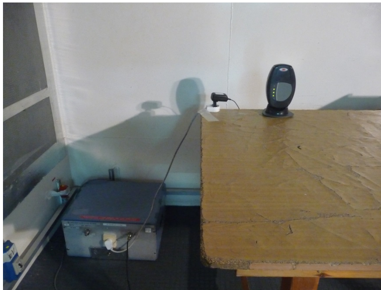
Photograph 7.4.1 Setup for conducted emission measurements
