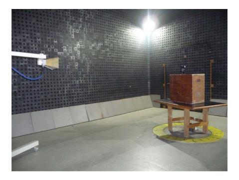
Photograph No.4 Setup for carrier and spurious emission field strength measurements, EUT close view
