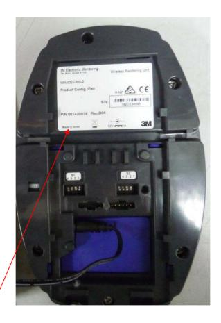
Label with FCC ID:LSQ-IDEU-830-2 is located at the rear side of the unit. The statement according to FCC part 15 §15.19(a)(3) is placed in User's Guide, page 57 (Application exhibit User\_manual\_27870).
