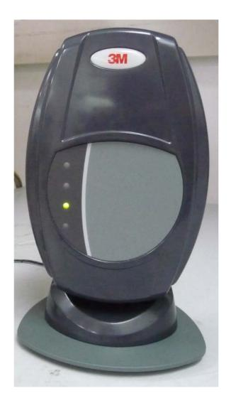
Photograph No.1 One-Piece Home Curfew RF Monitoring unit front view
