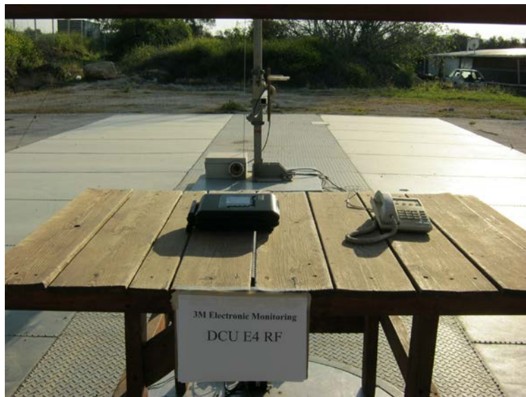
Figure 5. Radiated Emission Test Above 1000 MHz
