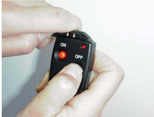
Figure 7 Disconnecting the Transmitter
