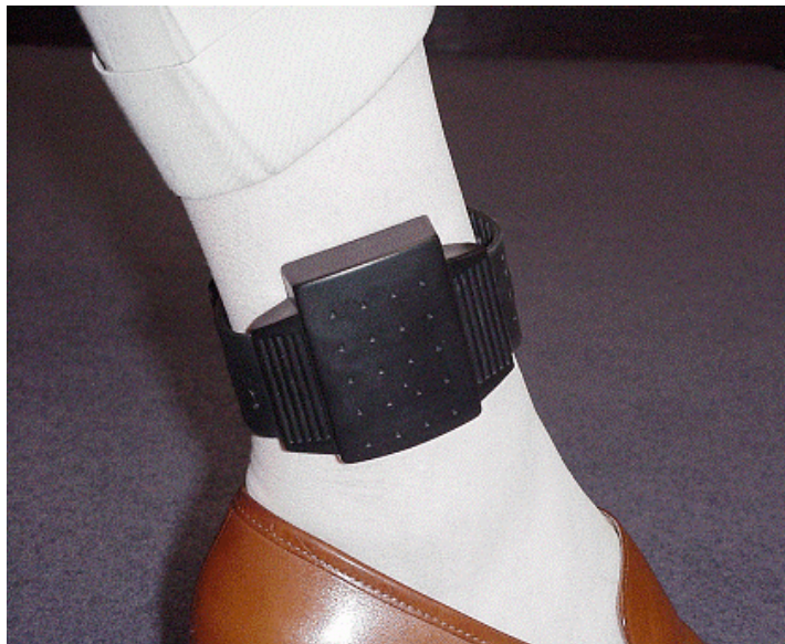
Figure 5 Protruding side of Transmitter directed upwards
