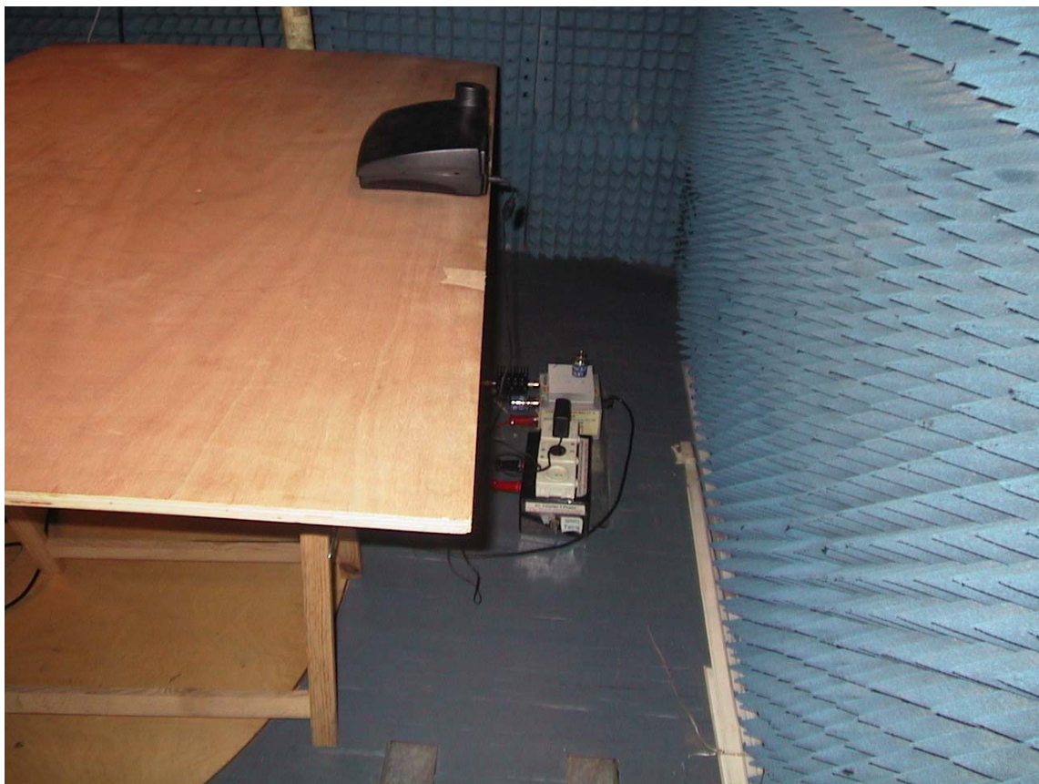
Conducted Emission, AC Power Leads Testing Setup
