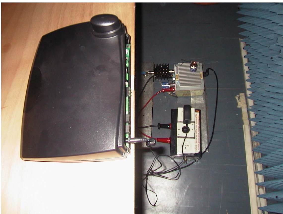
Conducted Emission, AC Power Leads Testing Setup
