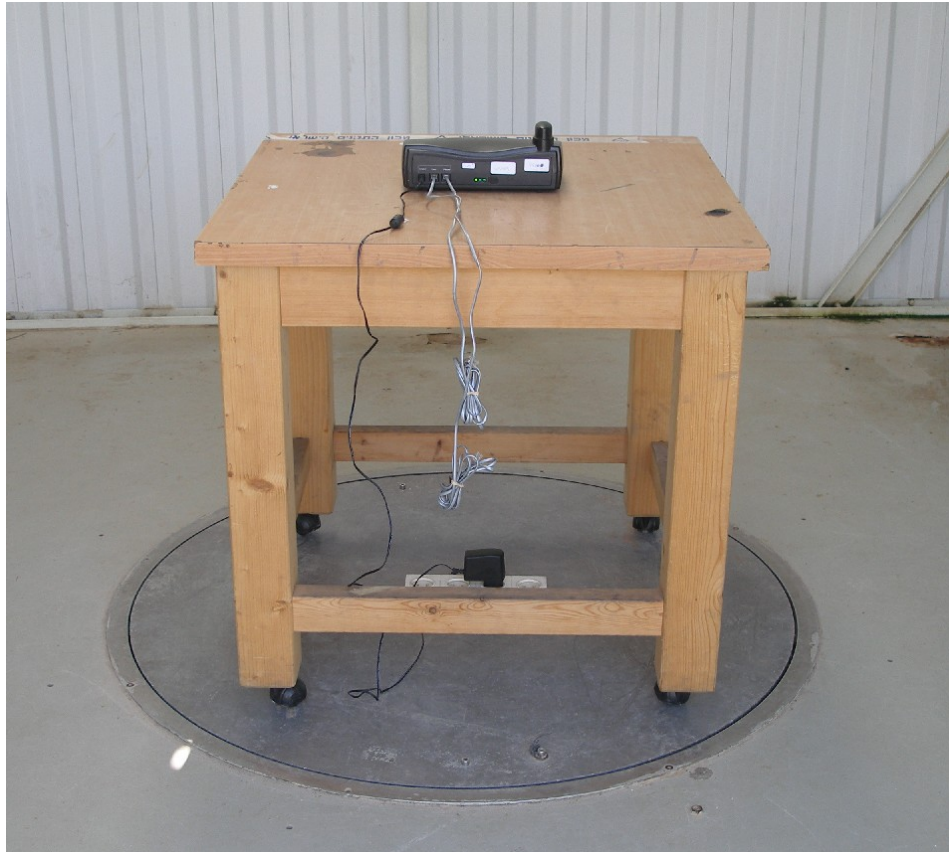
Photo # 2. Radiated emission test setup Rear view
