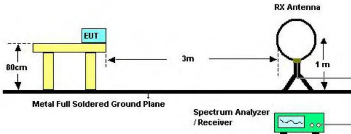
(B) Radiated Emission Test Set-Up Frequency 30 MHz~1 GHz
