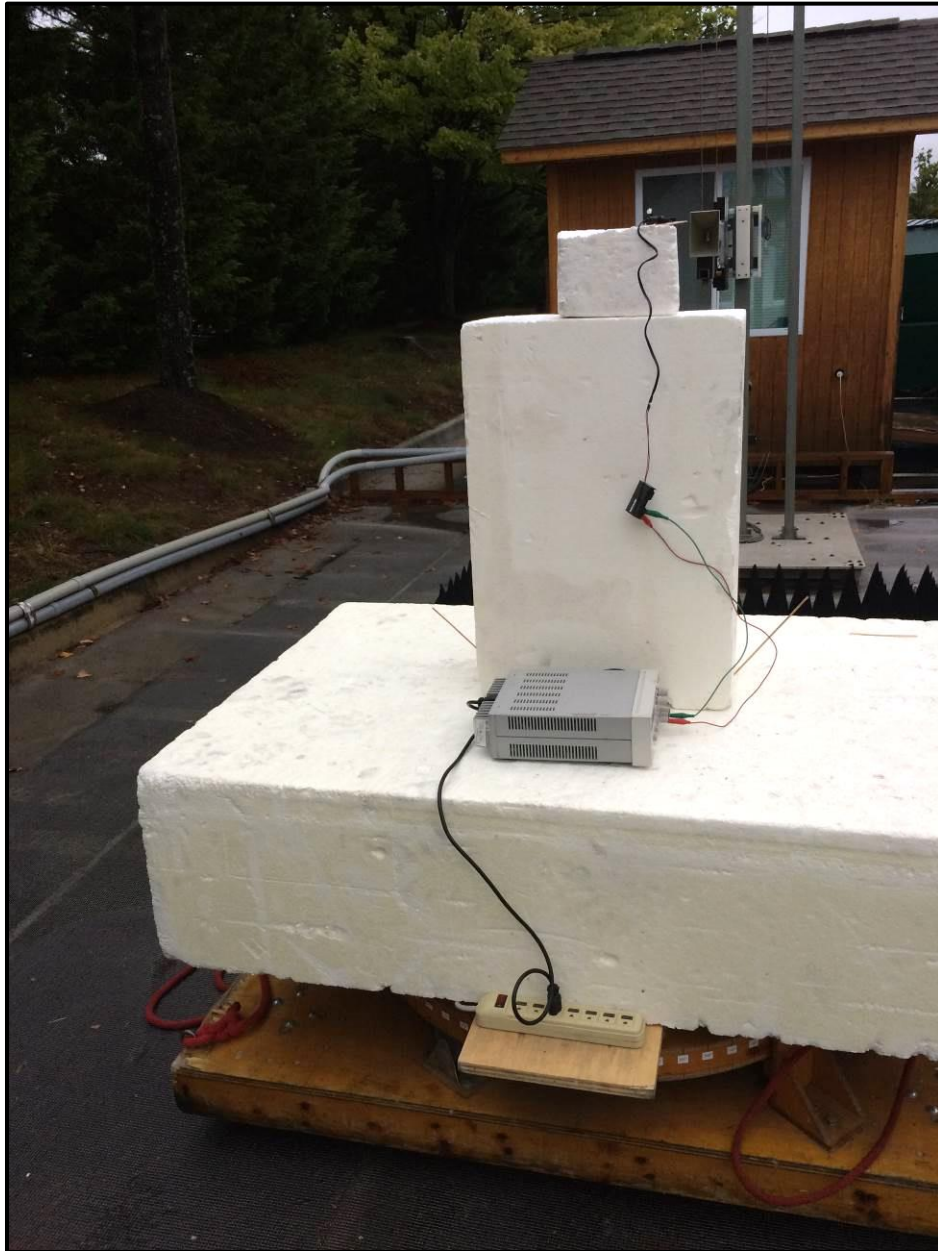
Photograph 5: Radiated Emissions Testing – Back View (> 1 GHz)
