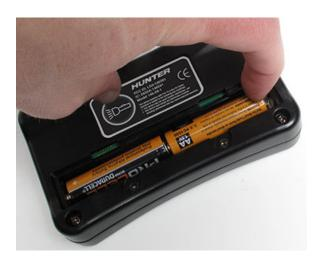
Replace the batteries with two new "AA" size batteries, making sure to observe the correct polarity.
