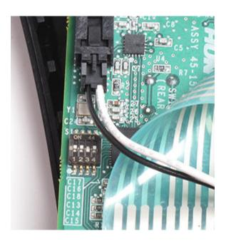
Set the dip switches in sequence for the desired channel using the table below.
