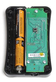
Remove the batteries from the device, then remove the three screws securing the main board.Gently turn the board over to access the dip switches on the opposite side.
