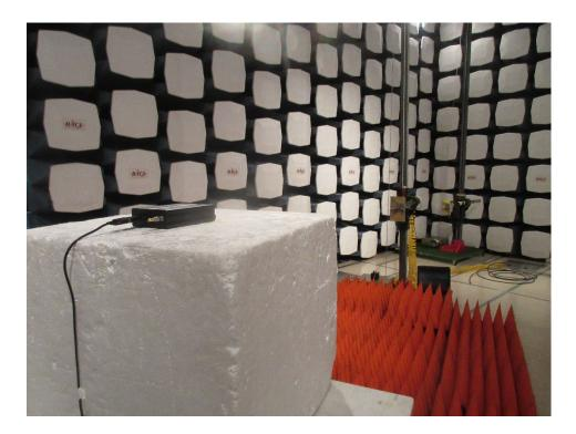
Radiated Emission above 1 GHz – Rear View
