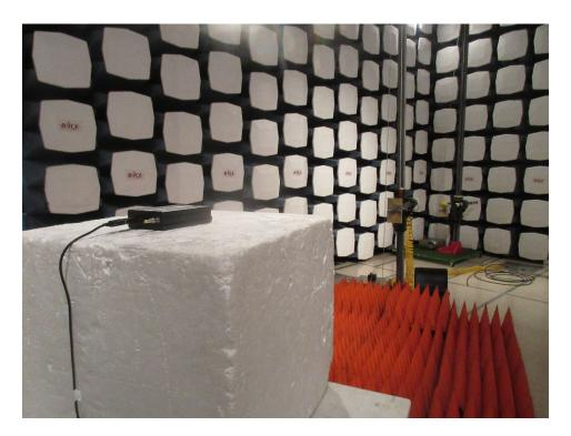
Radiated Emission above 1GHz - Rear View
