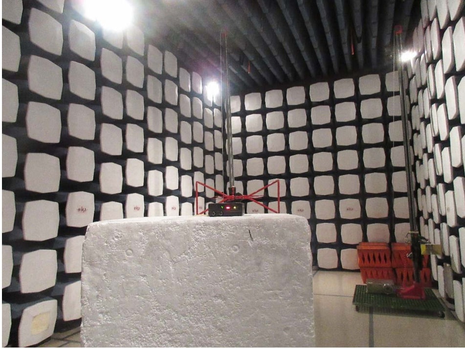
Radiated Emission below 1 GHz (SVR-300M) – Front View
