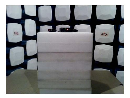
13.2 Below 1 GHz Radiated Emission – Rear View
