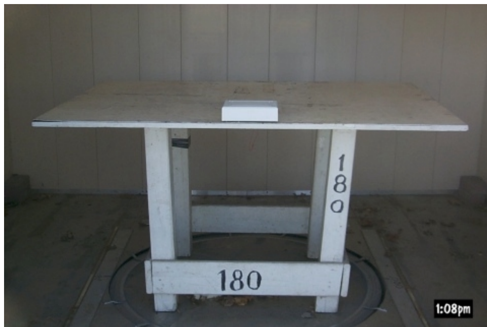
Figure 3.2 Radiated Test Setup, Rear View
