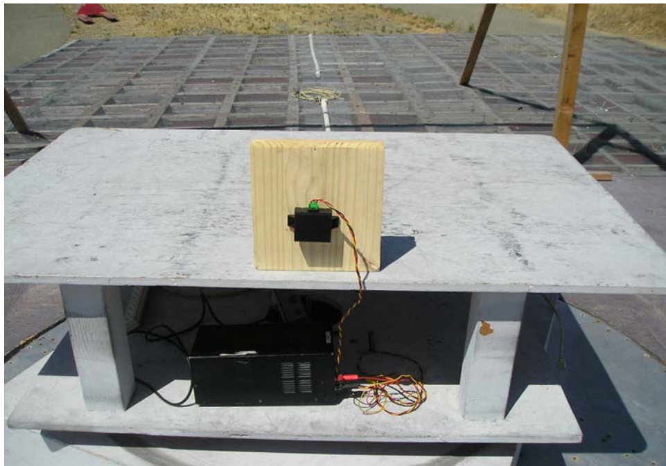
Figure 2: Open Field radiated Emissions Test Setup below 1GHz (View 2)
