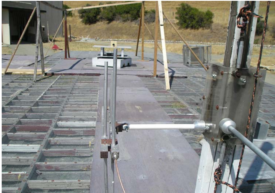
Figure 1: Open Field Radiated Emissions Test Setup below 1 GHz (View 1)
