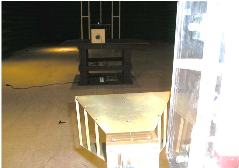
Figure 5 Test Set Up Photos – Field Strength of Fundamental Measurement
