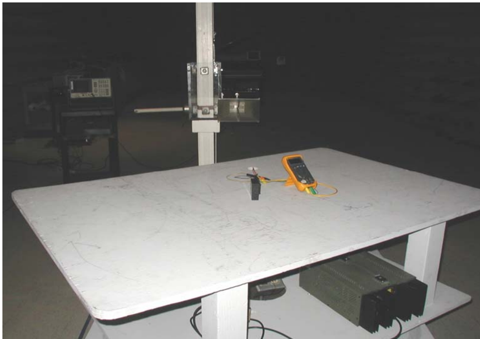
Figure 4: Maximized Radiated Emissions @ 1meter (above 18 GHz)
