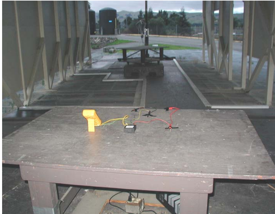
Figure 1: Maximized Radiated Emissions (below 1 GHz) – Front
