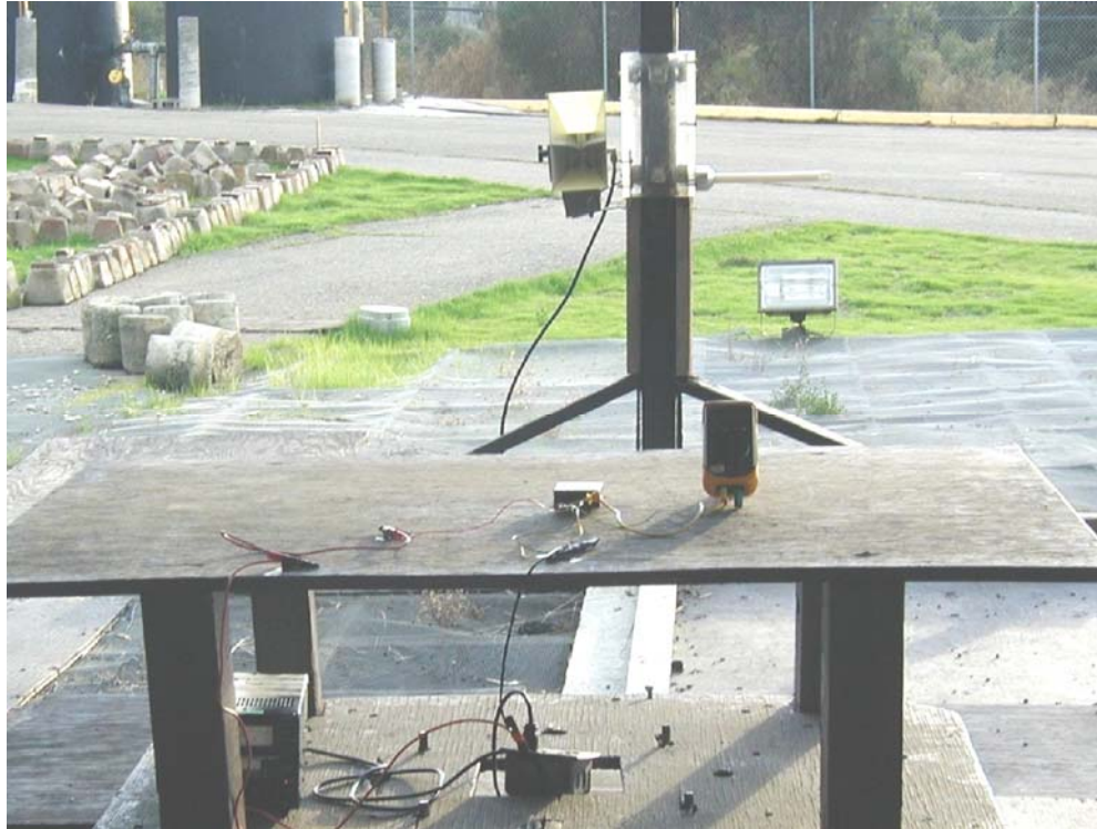
Figure 3: Maximized Radiated Emissions @ 3 meters (above 1 GHz)
