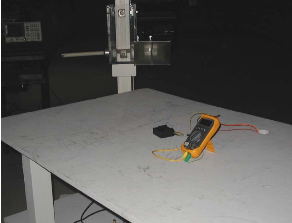
Figure 9: Test Set Up Photos – Spurious, Harmonics, and Restricted Bands Test Setup @ 1 meter
