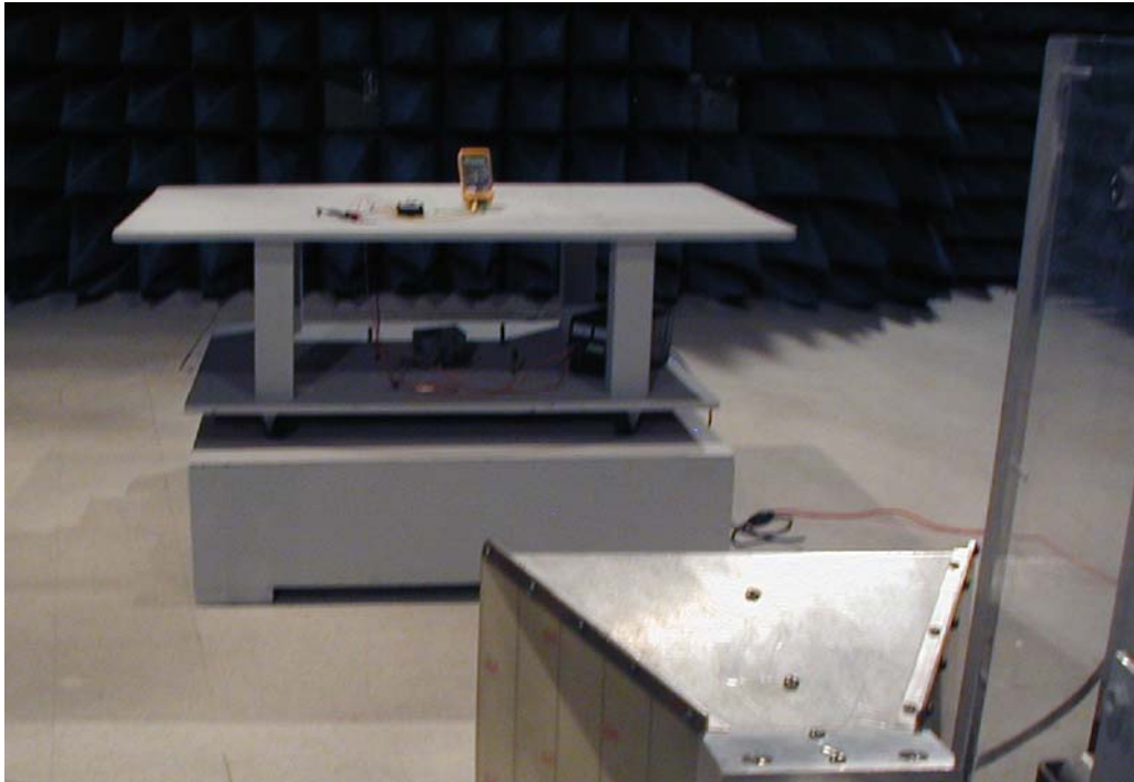
Figure 7 Test Set Up Photos – Field Strength of Fundamental Measurement (Front)
