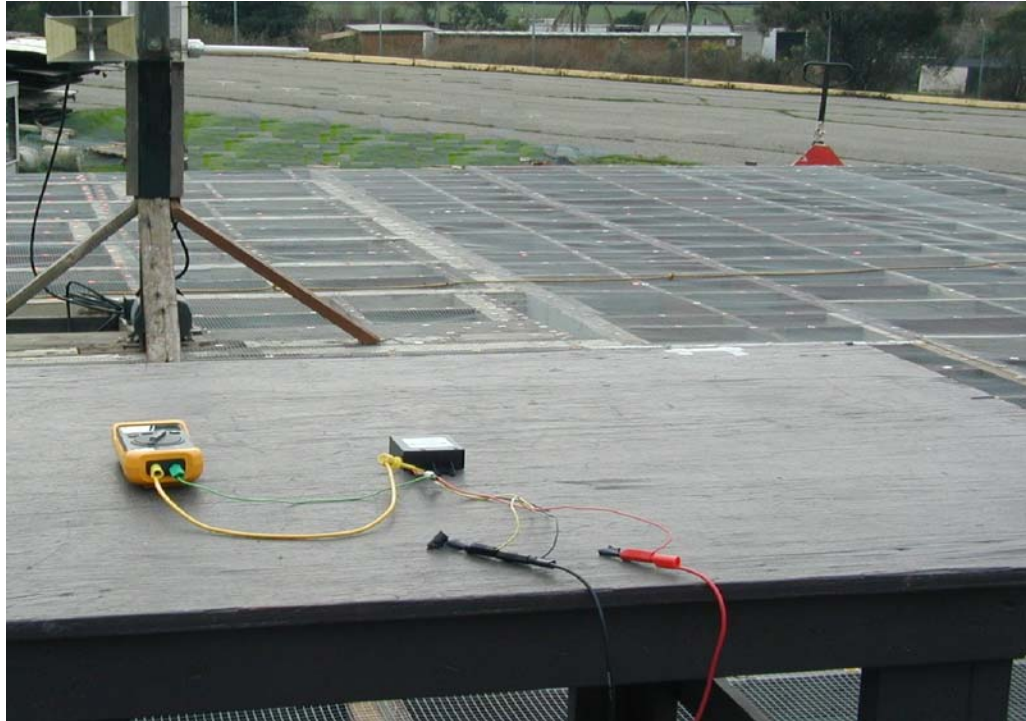
Figure 10: Test Set Up Photos – Spurious, Harmonics, and Restricted Test Set up (above 1GHz)
