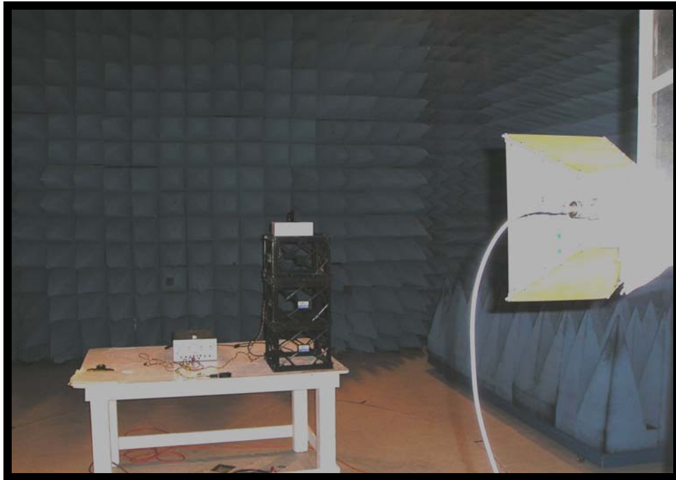
Figure 11: Spurious emission above 1 GHz (front view)
