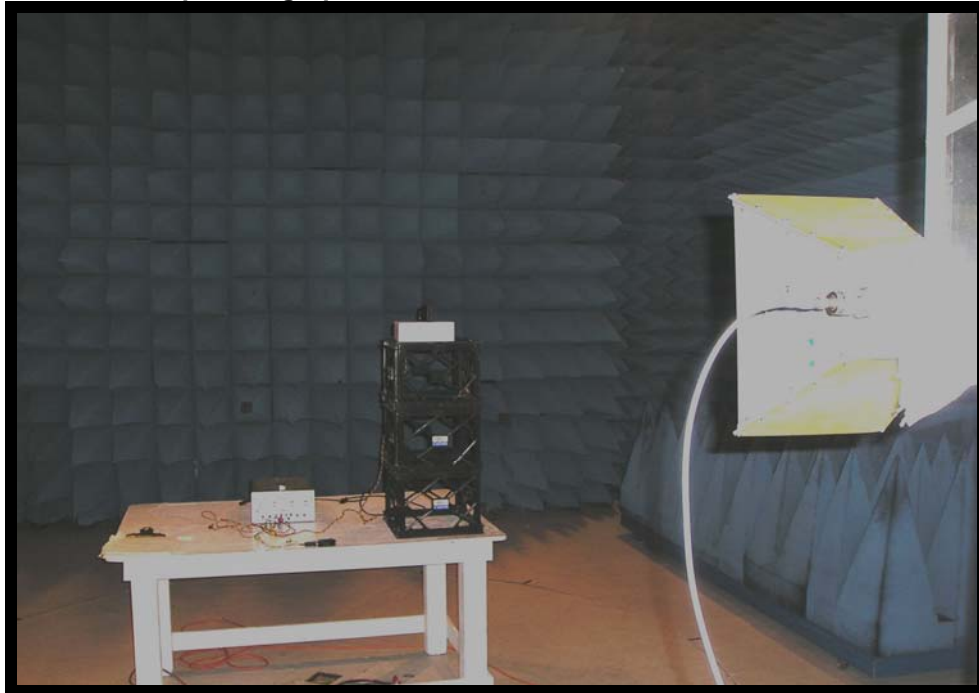
Figure 3: Radiated Emissions above 1 GHz (front view)
