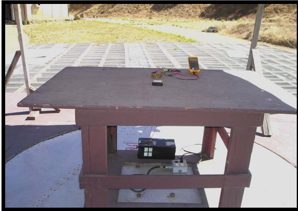
Figure 1: Open Field Radiated Emissions below 1 GHz (front view)
