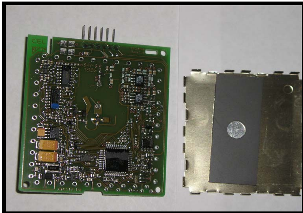
Figure 18: EUT Component View with shield off
