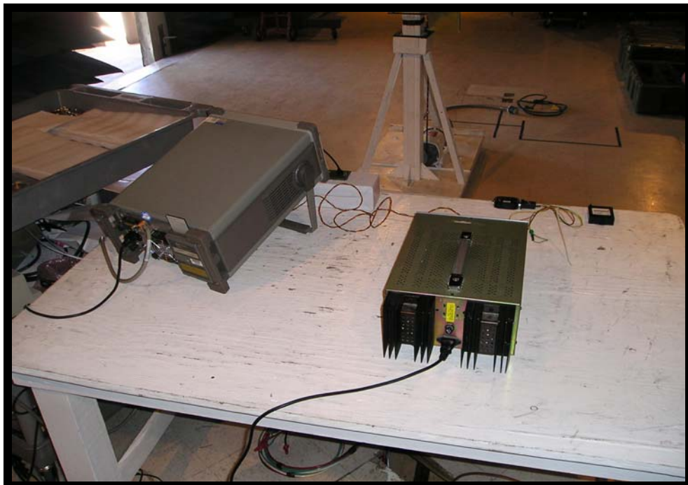
Figure 8 Test Set Up Photos – Field Strength of Fundamental Measurement (Rear)
