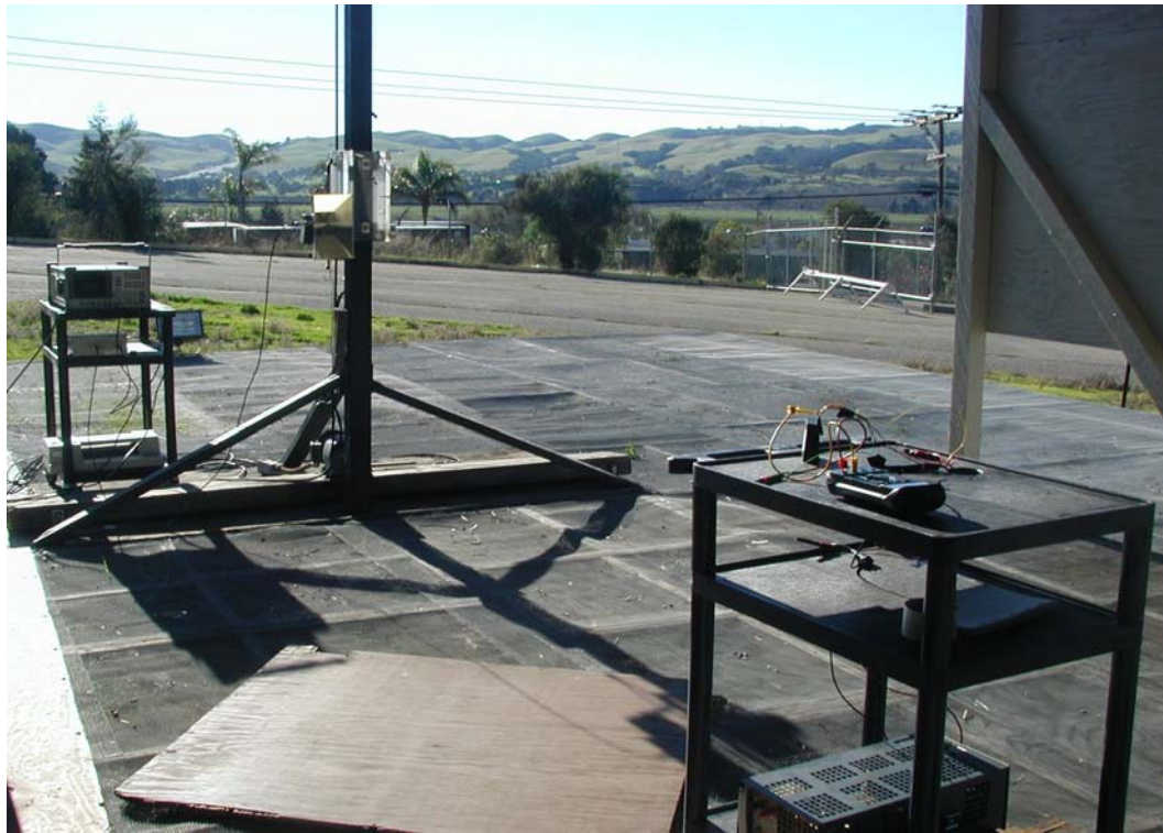
Figure 3 Radiated Emissions Test Setup – above 1GHz (OATS)
