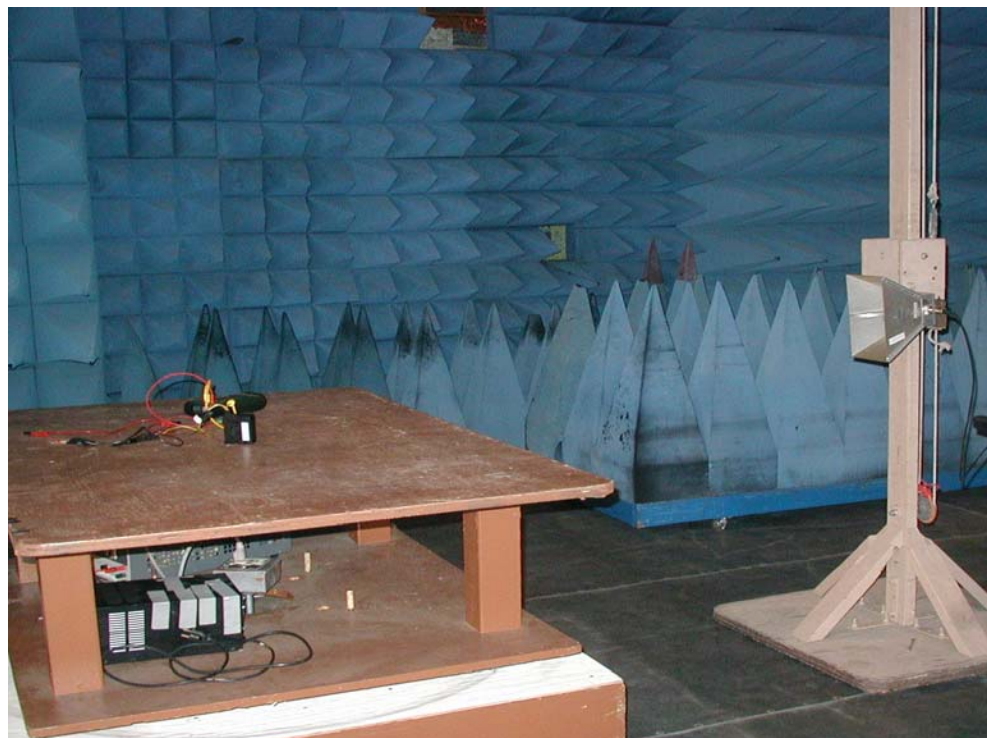
Figure 2 Radiated Emissions Test Setup – above 1GHz (Anechoic Chamber)
