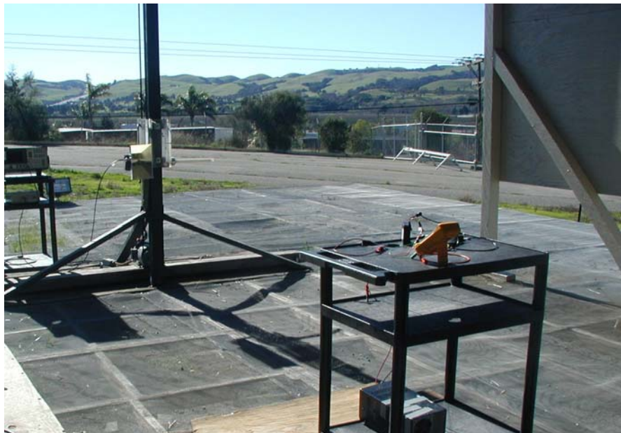
Figure 5 Test Set Up Photos – Field Strength of Fundamental Measurement (OATS)
