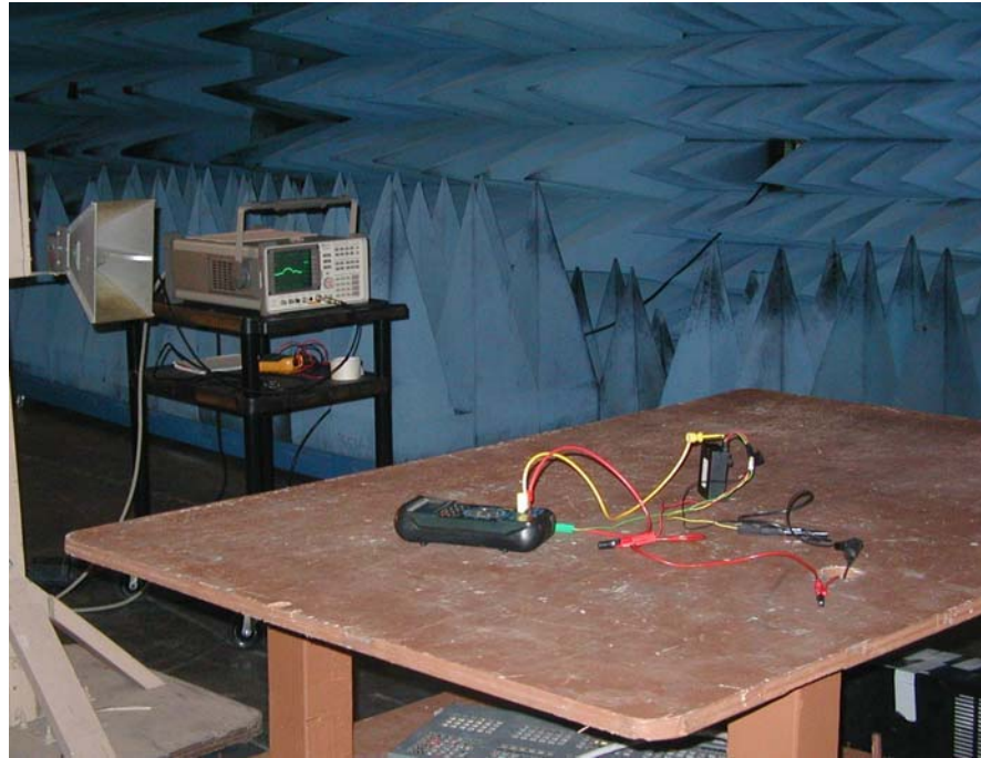
Figure 4 Test Set Up Photos – Field Strength of Fundamental Measurement (Anechoic Chamber)
