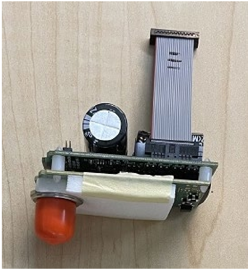
RF board, Analog board, Waveguide assembly side view
