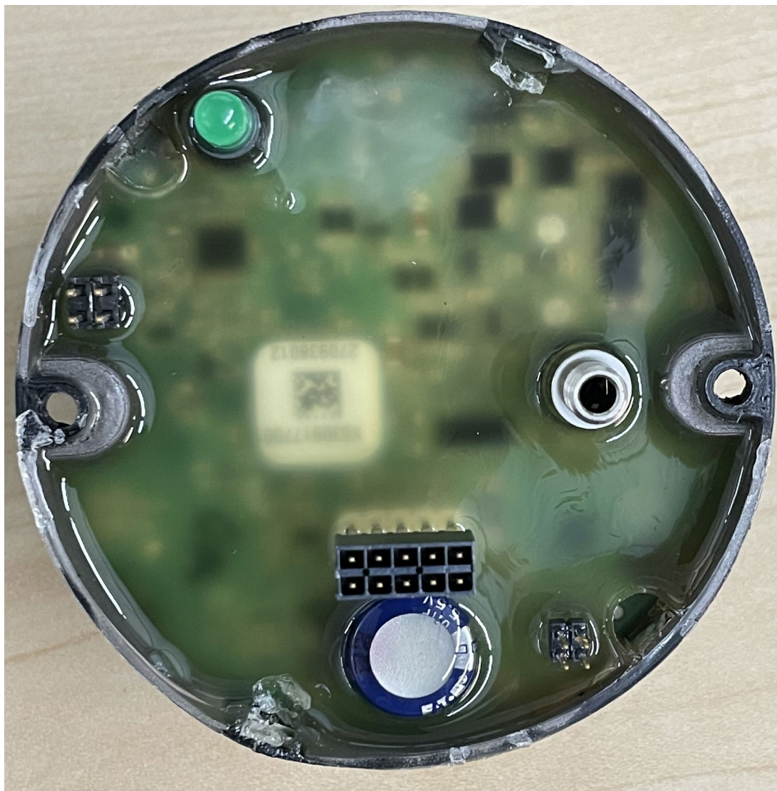
Digital Board and Potting cup assembly top view after potting without cover
