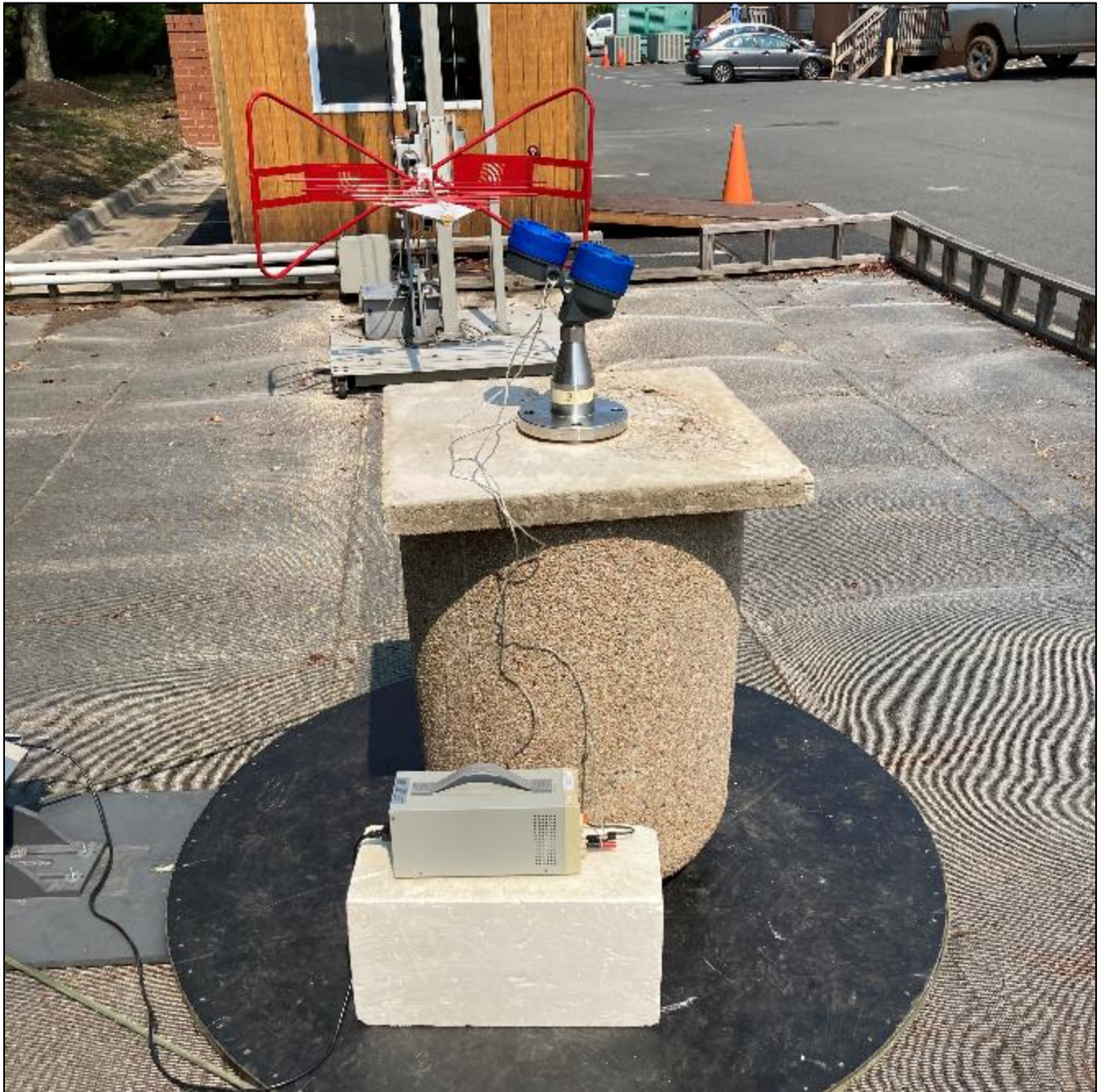
Photograph 4: Radiated Emissions – Concrete Container - Rear View
