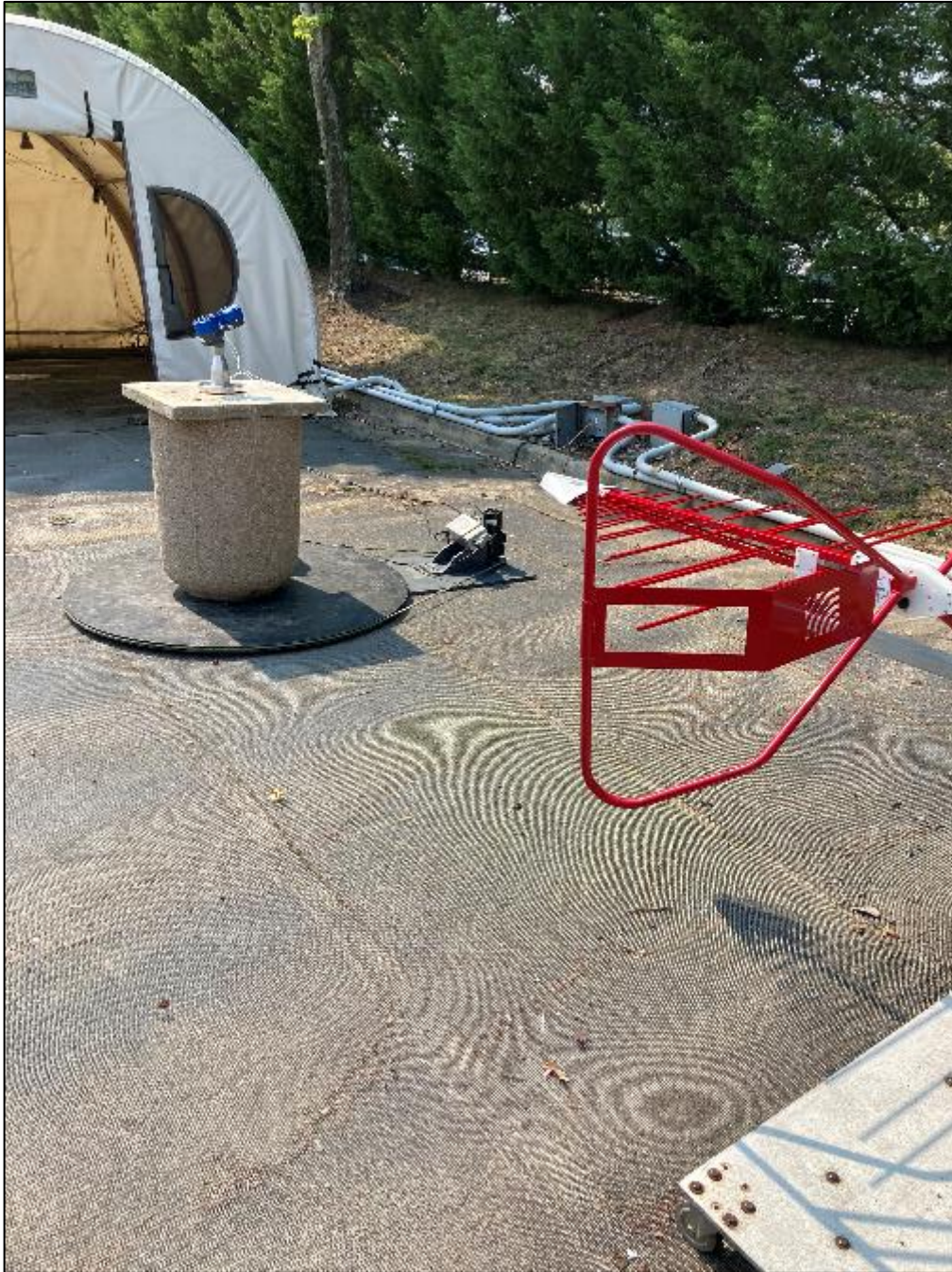
Photograph 3: Radiated Emissions – Concrete Container - Front View
