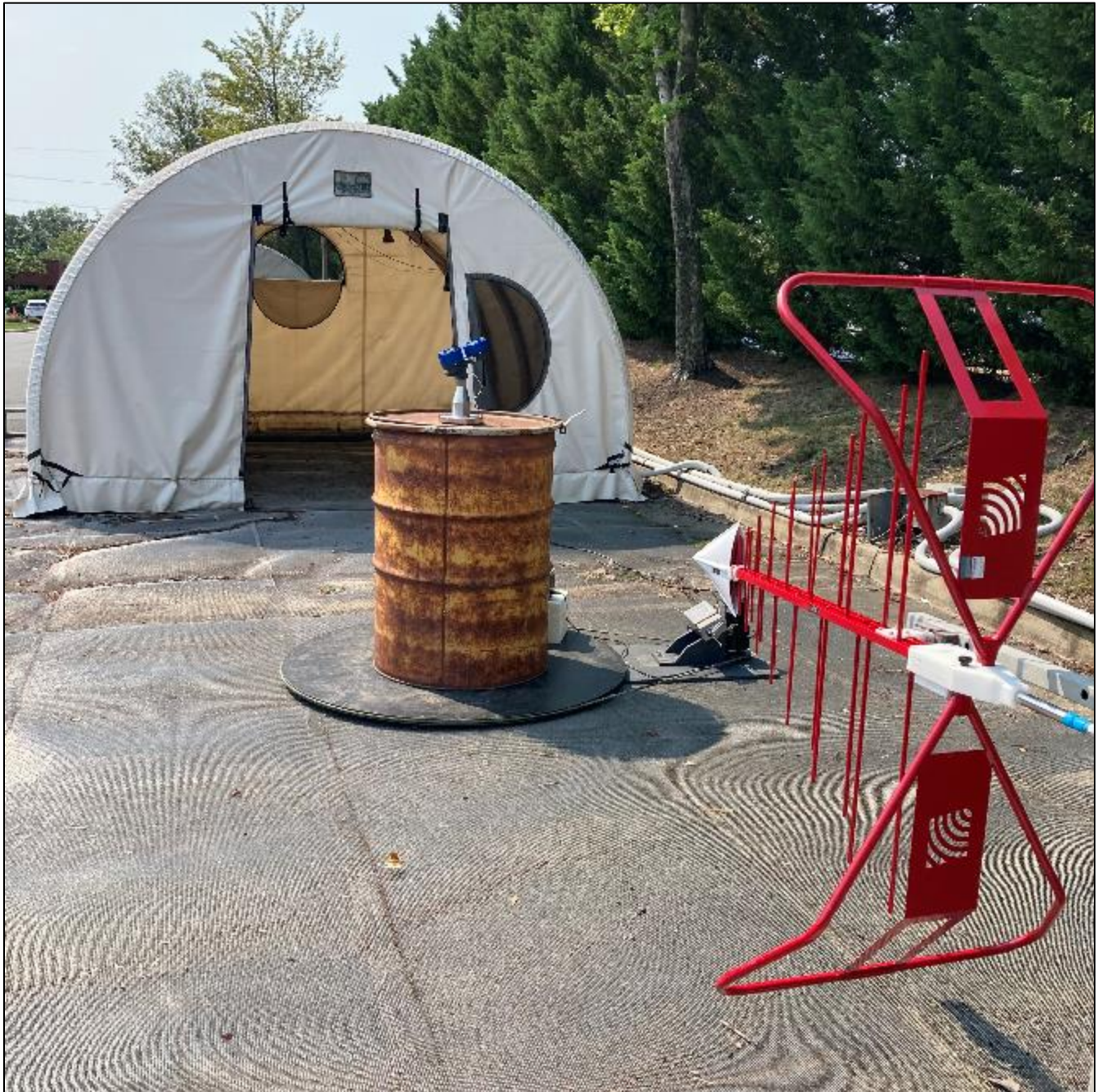
Photograph 5: Radiated Emissions – Metal Container - Front View
