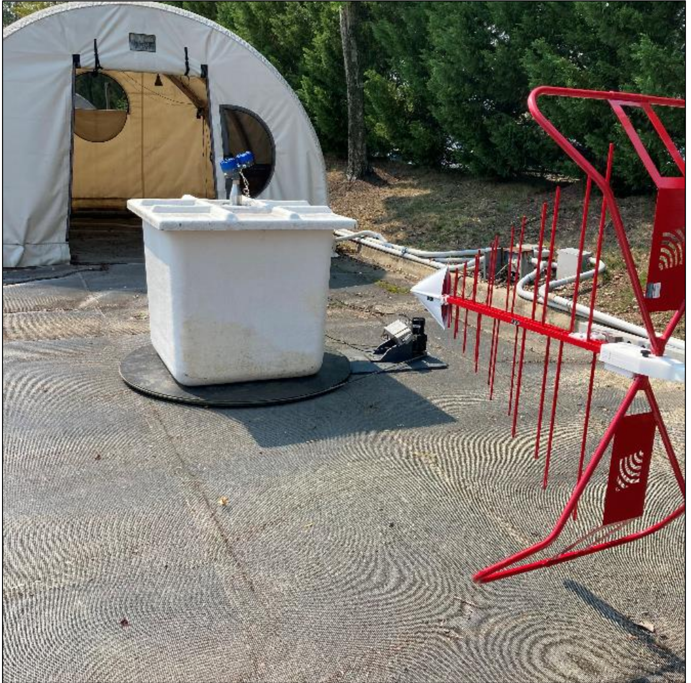
Photograph 7: Radiated Emissions – Fiberglass Container - Front View
