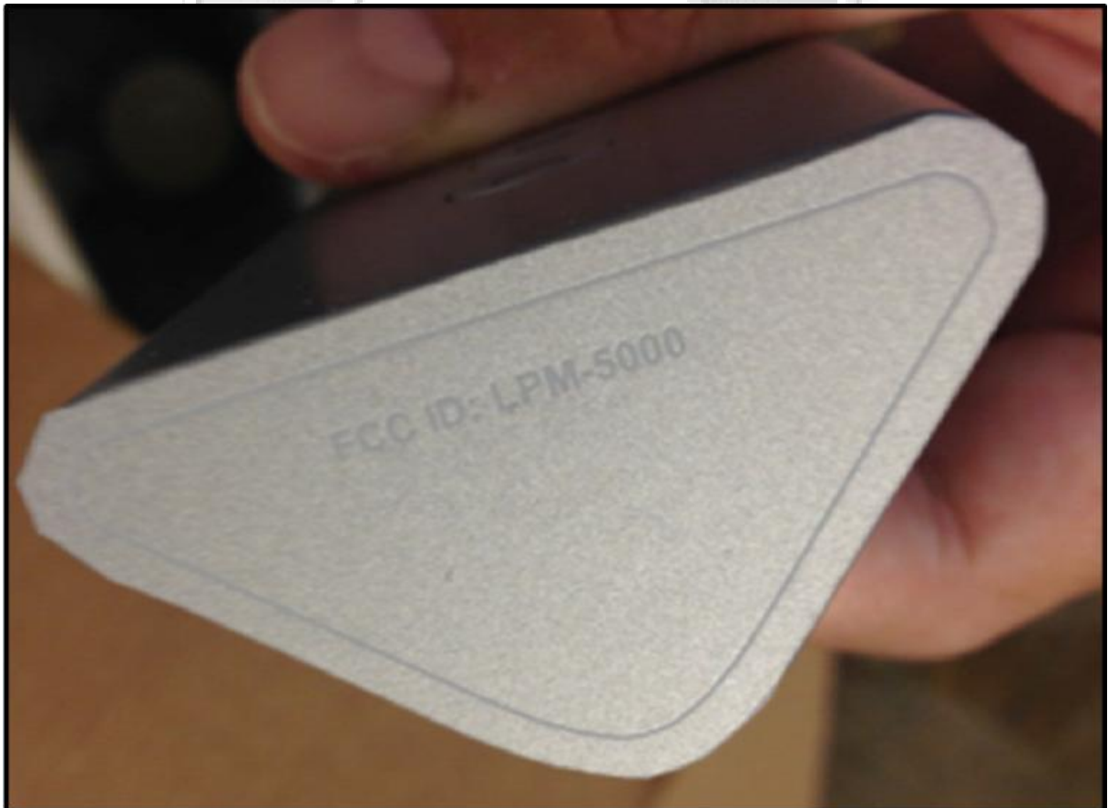
Physical Location of FCC Label on EUT
