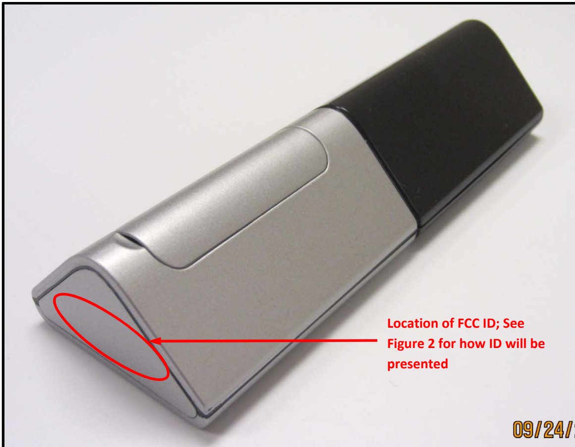
Figure 1 - Assembled remote looking from bottom showing location where FCC ID will be embedded in the in-mold label
