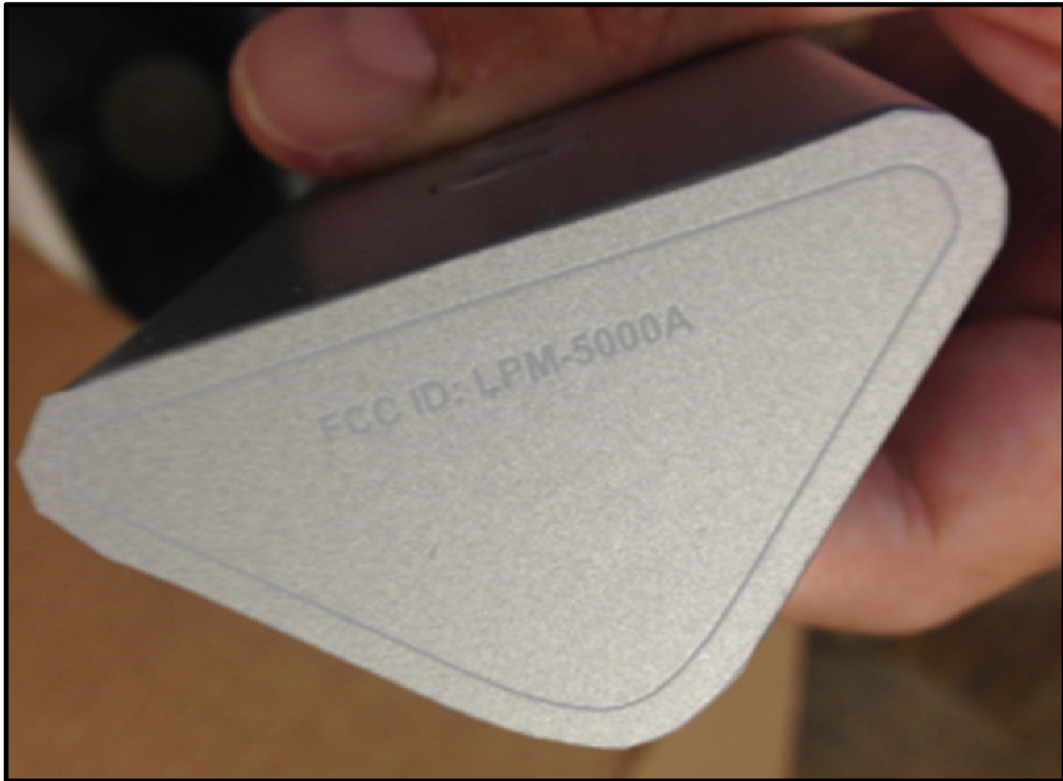
Figure 2 - Detail showing how FCC ID will be embedded in the in-mold label on the bottom cap of the remote. Remote ID will be LPM-5000B.
