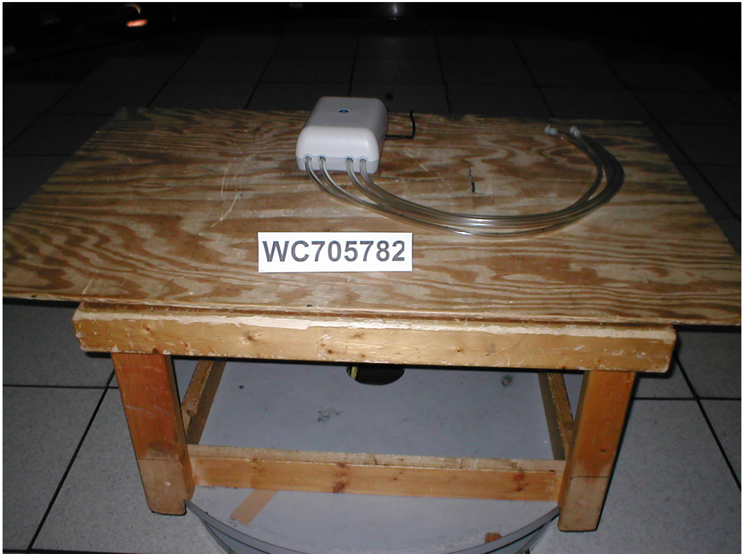
Test-setup photo, radiated emissions
