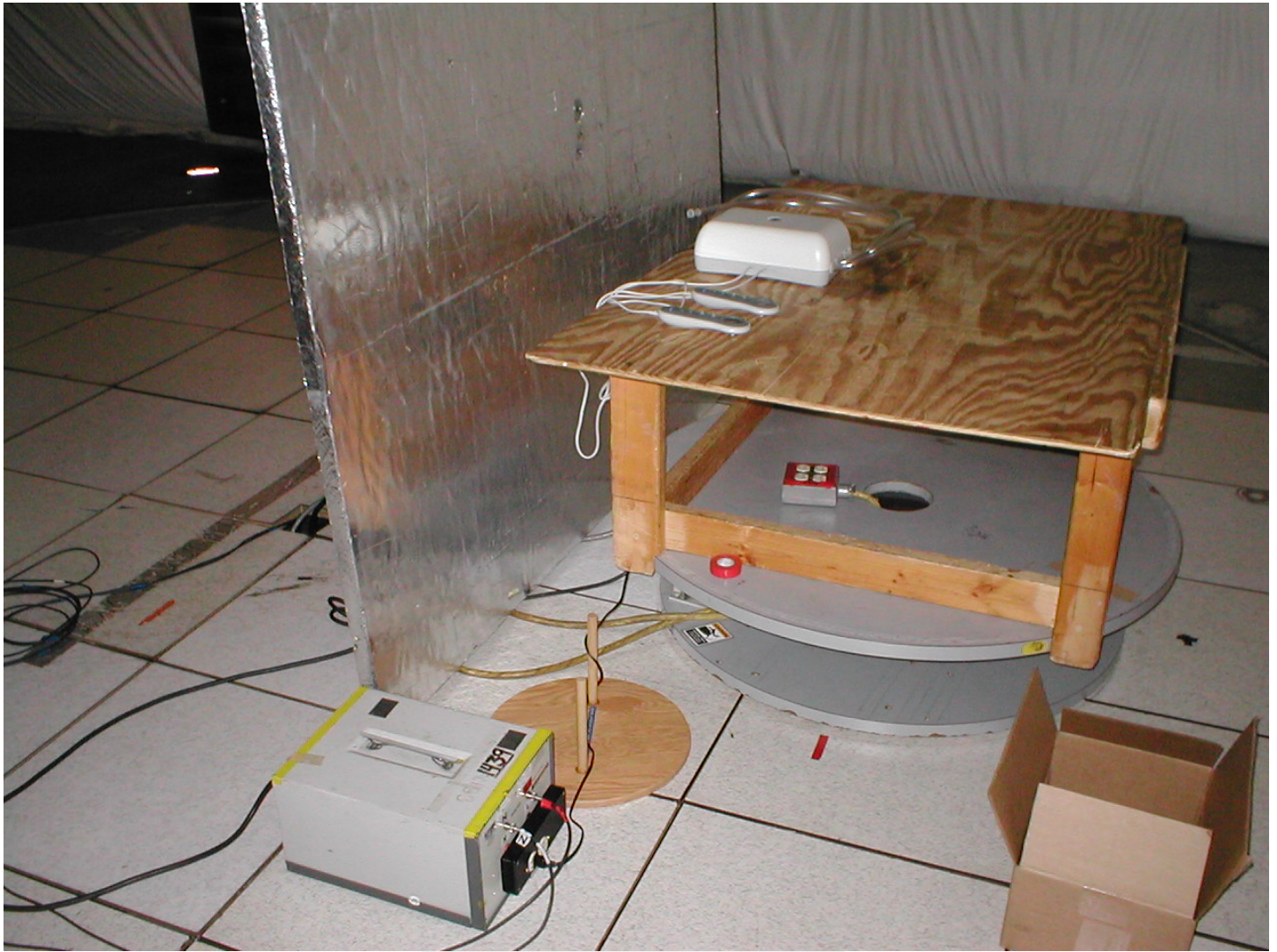
Test-setup photo, radiated emissions
