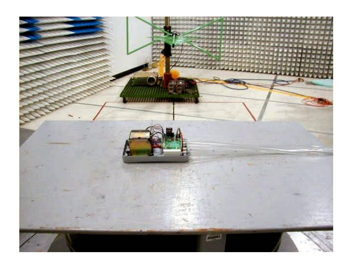
**Radiated Emissions Test Configuration**
