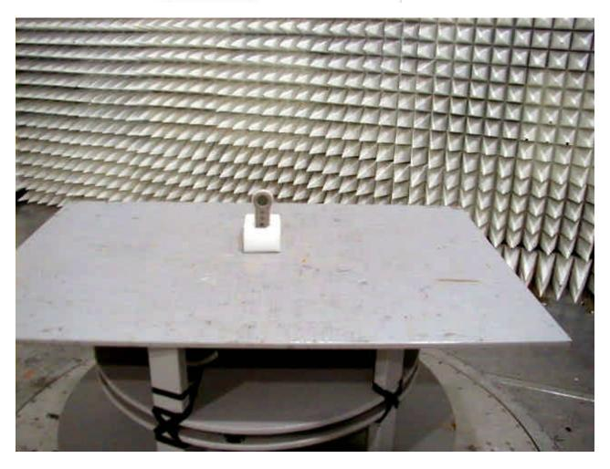
**Radiated Emissions Test Configuration**
