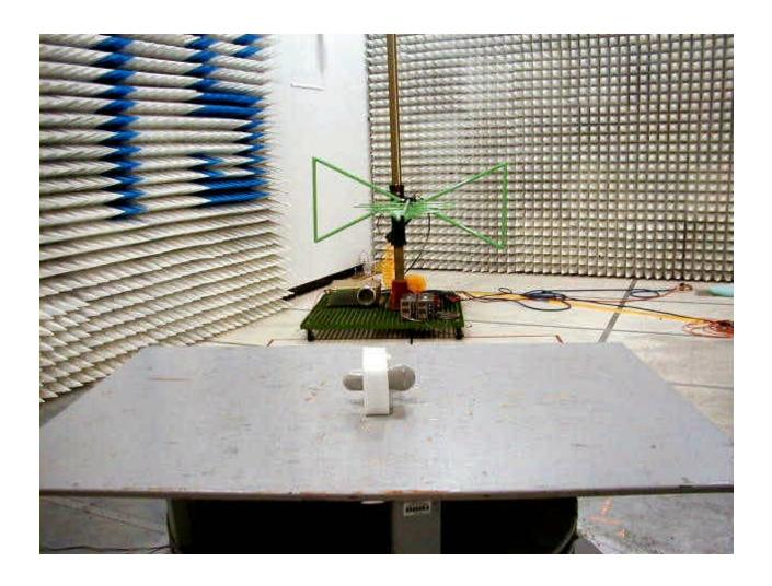
**Radiated Emissions Test Configuration**
