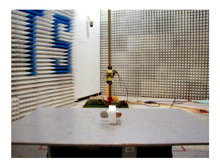
**Radiated Emissions Test Configuration**
