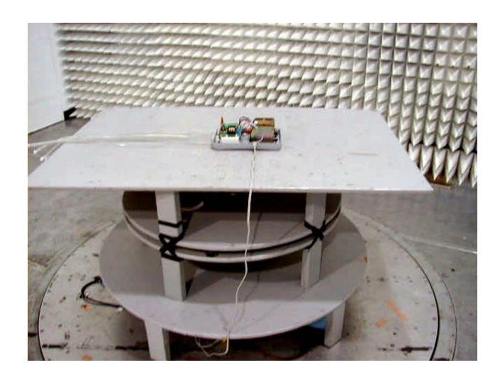
**Radiated Emissions Test Configuration**
