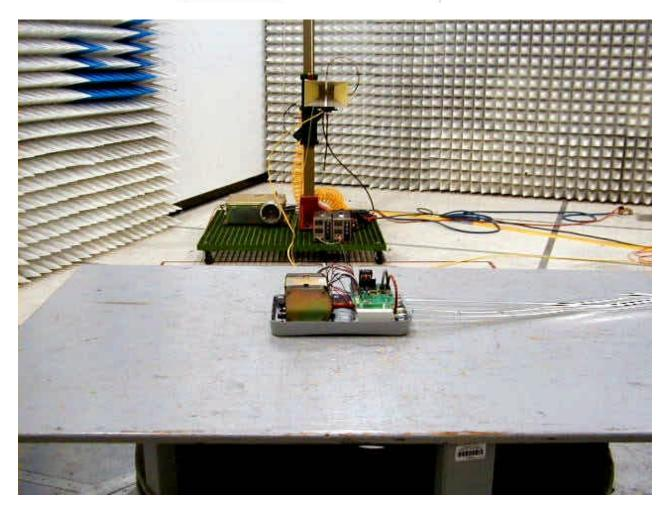
**Radiated Emissions Test Configuration**
