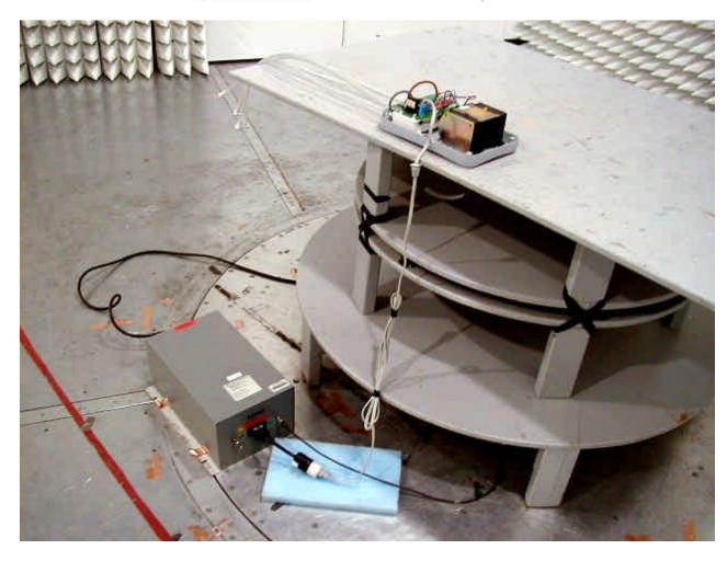
**Conducted Emissions Test Configuration**
