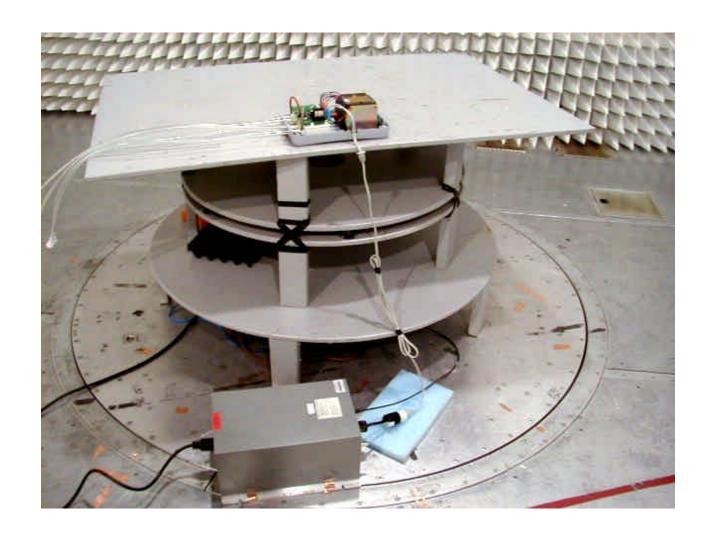
**Conducted Emissions Test Configuration**
