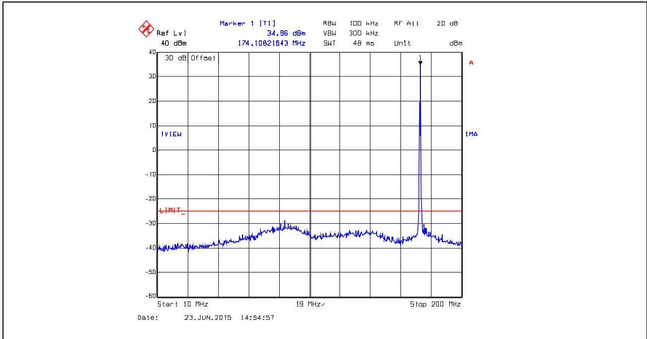
Plot 5.5.4.19. Conducted Transmitter Spurious Emissions, 173.9 MHz, High Power, 10 MHz – 200 MHz
