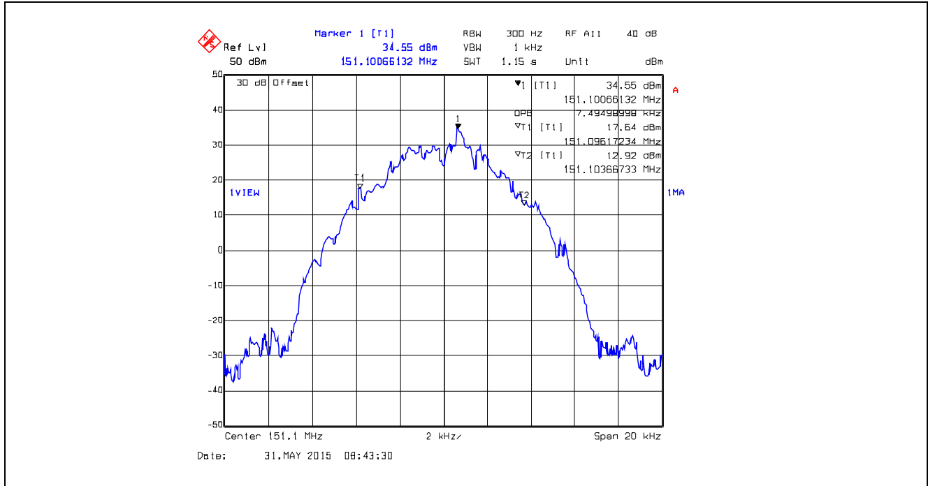
Plot 5.4.4.1.14. 99% Occupied Bandwidth, 12.5 kHz Channel Spacing, Digital 9.6 kbps, 151.1 MHz
