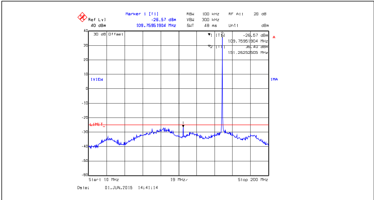
Plot 5.5.4.7. Conducted Transmitter Spurious Emissions, 151.1 MHz, High Power, 10 MHz – 200 MHz
