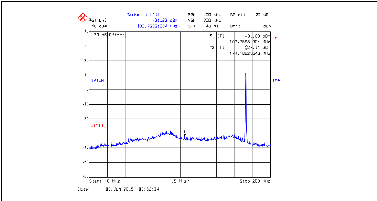
Plot 5.5.4.22. Conducted Transmitter Spurious Emissions, 173.9 MHz, Low Power, 10 MHz – 200 MHz
