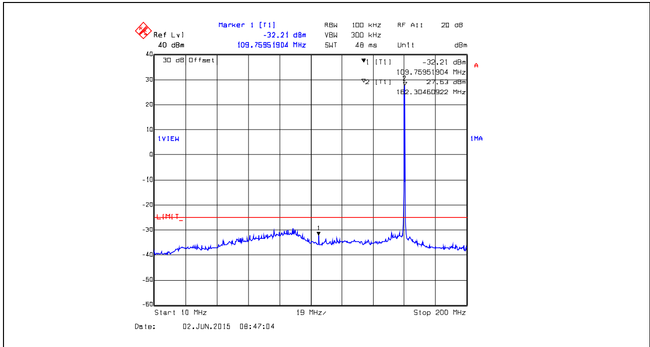
Plot 5.5.4.16. Conducted Transmitter Spurious Emissions, 162.0 MHz, Low Power, 10 MHz – 200 MHz
