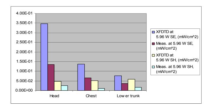
In summary, the aggregated data presented in this analysis show that the simulation model employed in the SAR compliance assessment relative to the in-vehicle exposure is consistently conservative.
