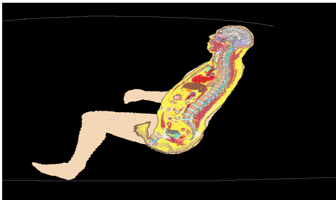
Figure 2: Passenger (back seat) model exposed to a trunk-mount antenna: XFDTD geometry. The antenna is mounted at 85 cm from the passenger located in the center of the back seat.
