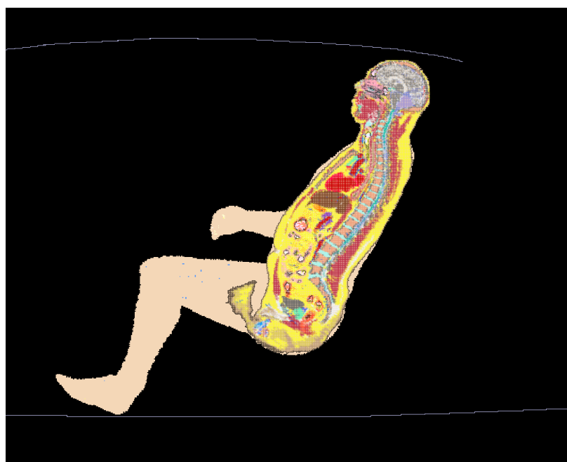
Figure 2: Passenger (back seat) model exposed to a trunk-mount antenna: XFDTD geometry. The antenna is mounted at 85 cm from the passenger located in the center of the back seat.
