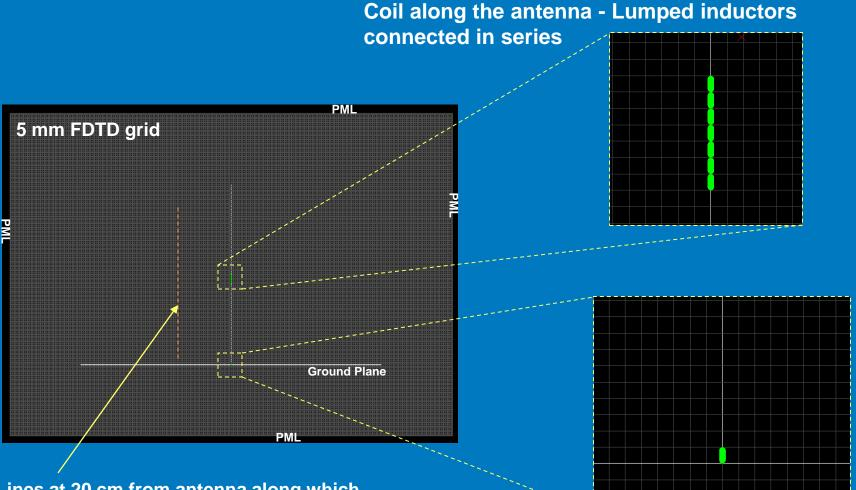
Lines at 20 cm from antenna along which the simulated and measured field values were compared
