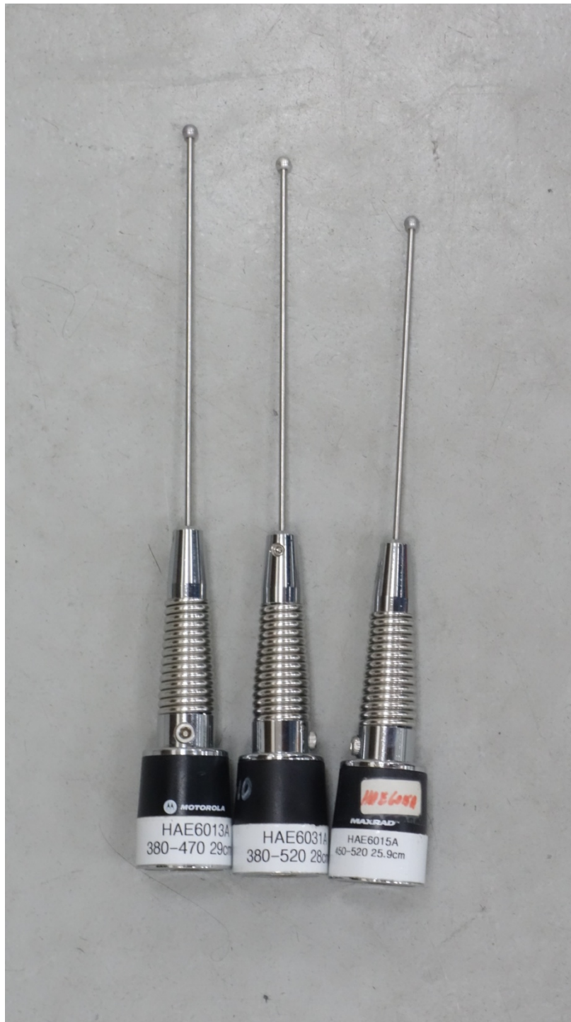
UHF Antenna kit numbers, from left to right; HAE6013A, HAE6031A and HAE6015A
