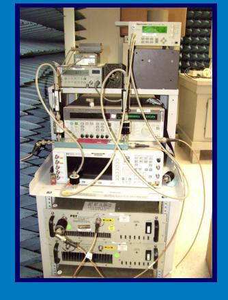
Antenna return loss was measured and taken into account in normalization of the results to 1.0 W radiated power
