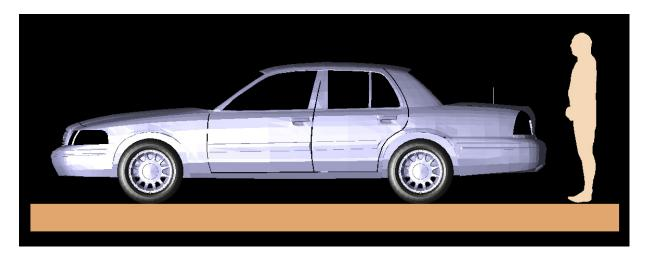
Centered bystander model at 20 cm from vehicle equipped with a trunk-mount quarter-wave monopole antenna operating at UHF (450 MHz).
