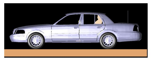
Passenger model in the center back-seat of vehicle equipped with a trunk-mount quarter-wave monopole antenna operating at VHF (150 MHz).
