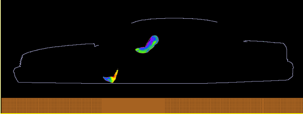
Figure 4. SAR distribution at 150.8 MHz in the driver model produced by the trunk mount HAD4007A antenna. The contour plot is relative to the plane where the peak 1-g average SAR for this exposure condition occurs.
