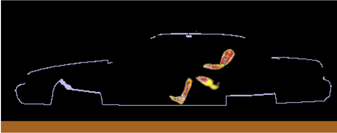
Figure 5. SAR distribution at 809.0125 MHz in the passenger model produced by the roof-mount HAF4013A antenna. The contour plot is relative to the plane where the peak 1-g average SAR for this exposure condition occurs.
