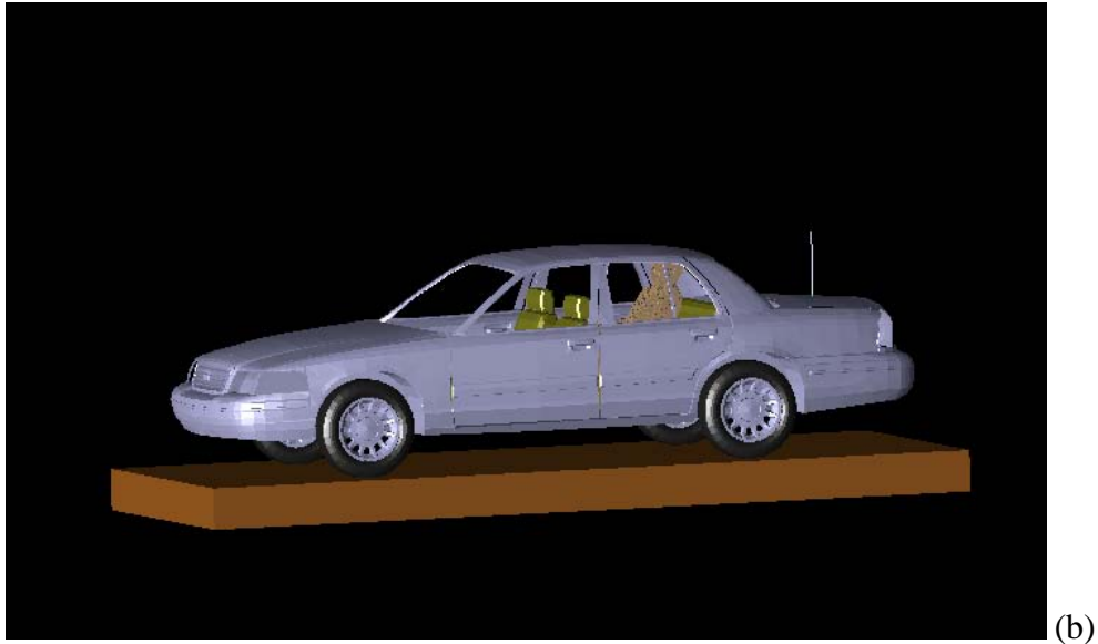
Figure 2: Passenger model exposed to roof mounted (a) and trunk-mounted (b) antennas: XFDTD geometry.
