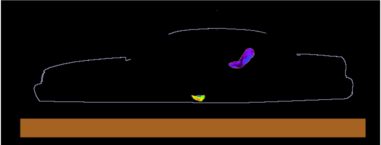
Figure 7. SAR distribution at 445.0125 MHz in the passenger model produced by the roof-mount HAE4011A antenna. The contour plot is relative to the plane where the peak 1-g average SAR for this exposure condition occurs.
