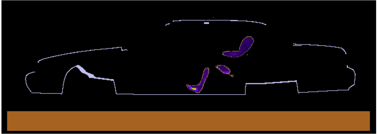
Figure 5. SAR distribution at 470.0125 MHz in the passenger model produced by the roof-mount HAE4004A antenna. The contour plot is relative to the plane where the peak 1-g average SAR for this exposure condition occurs.
