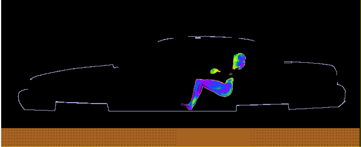
Figure 6. SAR distribution at 156.4 MHz in the driver model produced by the roof-mount HAD4008A antenna. The contour plot is relative to the plane where the peak 1-g average SAR for this exposure condition occurs.
