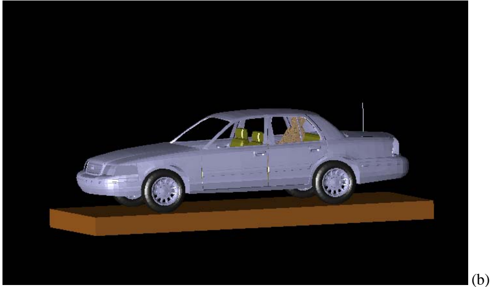
Figure 3: Passenger model exposed to roof mounted (a) and trunk-mounted (b) antennas: XFDTD geometry.
