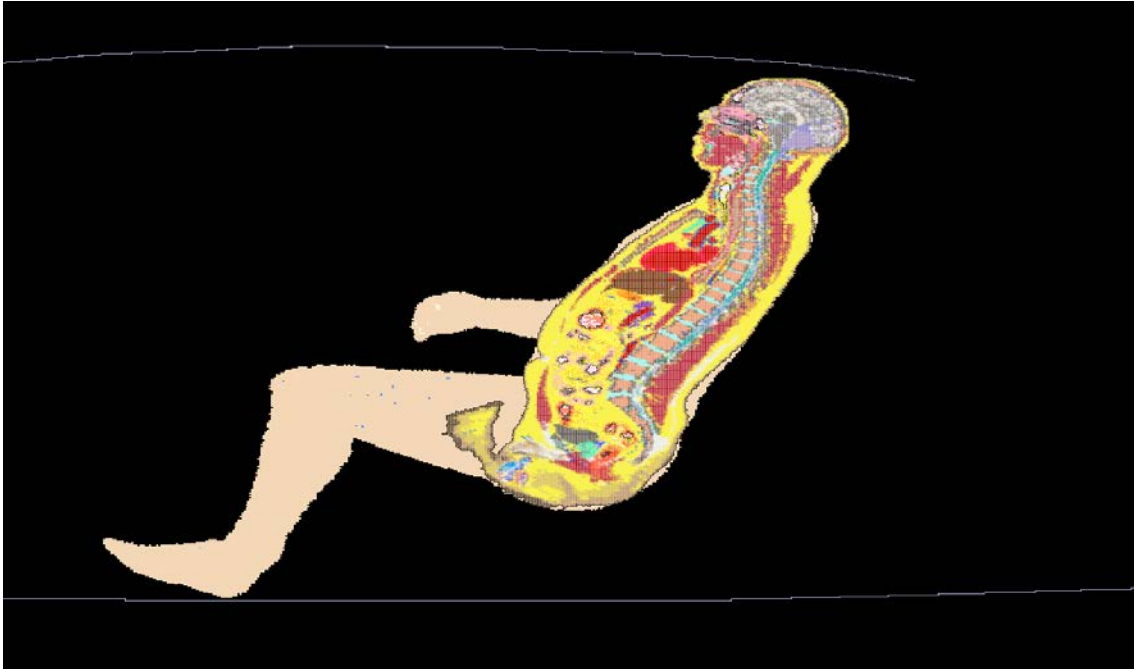
Figure 2: Passenger model exposed to a trunk-mount antenna: XFDTD geometry.
