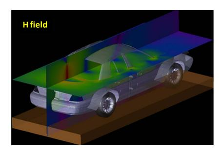
As done in the measurements, the equivalent power density (S) is computed from the E-field, the H-field being much lower. The following table reports the E-field values computed by XFDTD<sup>TM</sup> at the three locations, and the corresponding power density.
