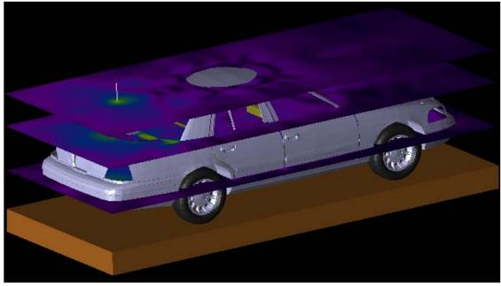
The equivalent power density (S) is computed from the E-field. The following table reports the E-field values computed by XFDTD<sup>TM</sup> at the three locations, and the corresponding power density.
