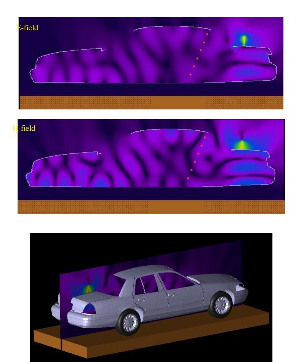
The equivalent power density (S) is computed from the E-field and the H-field separately. The following table reports the E-field values computed by  $XFDTD^{TM}$  at the six locations, and the corresponding power density.
