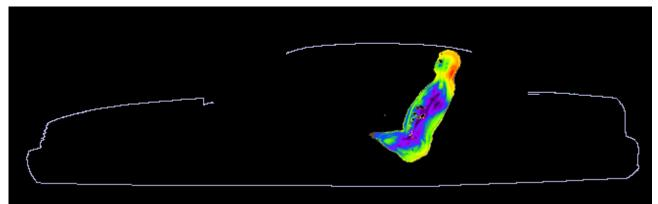
Figure 3. SAR distribution at 498.0000 MHz in the passenger back side model produced by the trunk mount HAD4004A antenna. The contour plot is relative to the plane where the peak 1-g average SAR for this exposure condition occurs.
