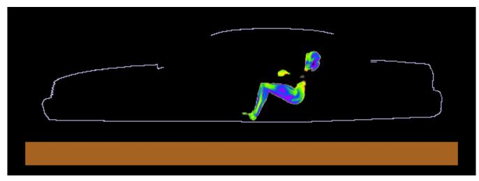
Figure 5. SAR distribution at 419.5 MHz in the passenger back center model produced by the trunk mount HAE6012A antenna. The contour plot is relative to the plane where the peak 1-g average SAR for this exposure condition occurs.
