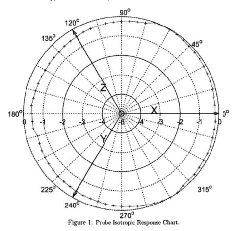
$\label{eq:source} Isotropic \ response \ is \ measured \ in \ a \ 20 \ V/m \ field \ at \ 400 \ MHz \\ * Isotropy \ is \ the \ maximum \ deviation \ from \ the \ geometric \ mean \ as \ defined \ by \ IEEE \ 1309-2005.$
